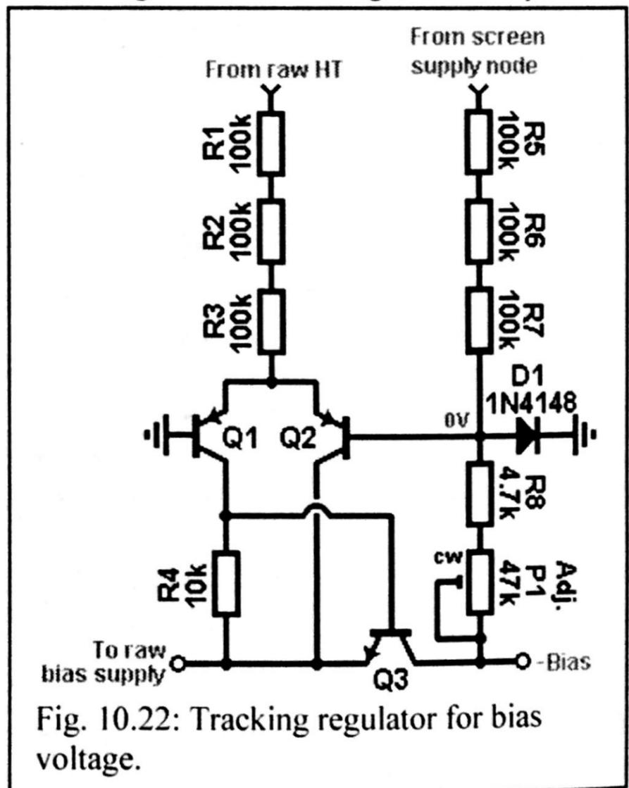
Fig. 10.22: Tracking regulator for bias voltage.
