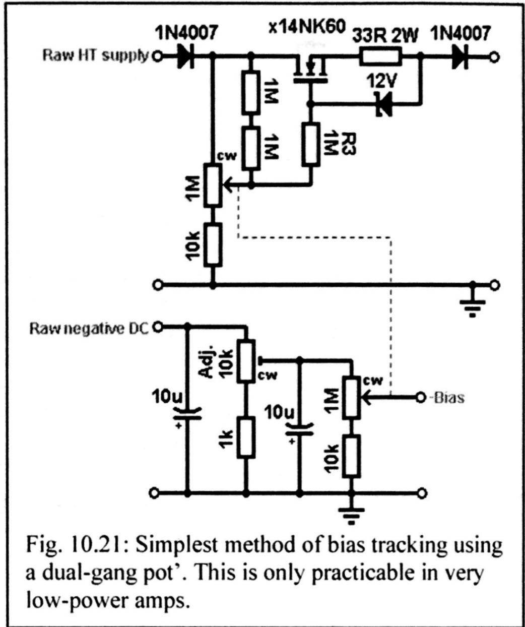
Fig. 10.21: Simplest method of bias tracking using a dual-gang pot'. This is only practicable in very low-power amps.
